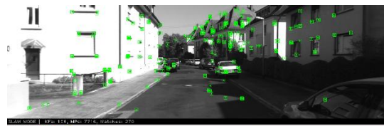
Figure 5. ORB Algorithm working with KITTI dataset [15].
